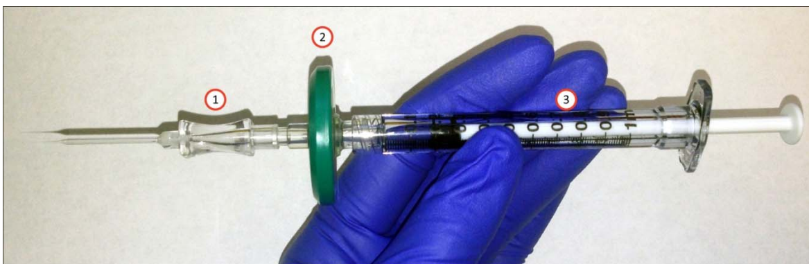
Figure 4: DCU and filter affixed to a luer lock sterile syringe. 1 – DCU; 2 – filter, 3 – syringe.
